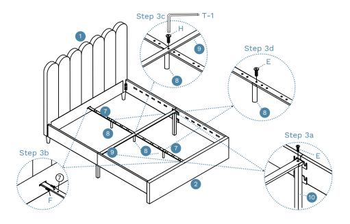
Step 3a: Attach Panel (10) to assembled frame as shown and secure with  $2\ x$  bolts (E).
