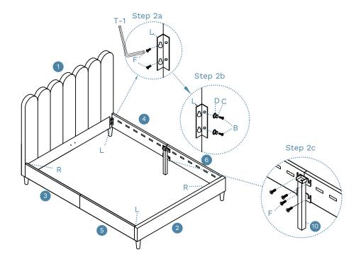
Attach 2 x left plates (L) and 2 x right plates (R) to panels [3], [4], [6] and [5] as shown in Step 2a and Step 2b and secure with 8 x bolts (F), 8 x bolts (B), 8 x spring washers (C) and 8 x washers (D).
