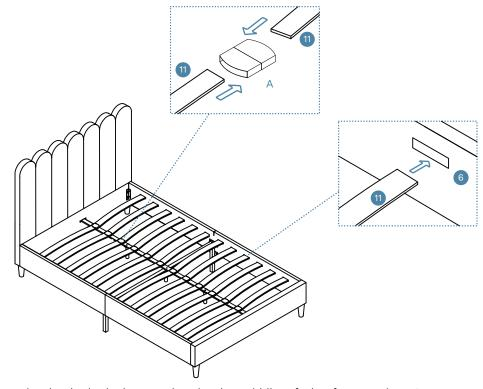
Join the bed planks together in the middle of the frame using 12x double caps (A). Insert the end of the planks into the bed frame as shown and attach the double caps (A) into panel [6]. Make sure the double caps (A) click securely into place.
